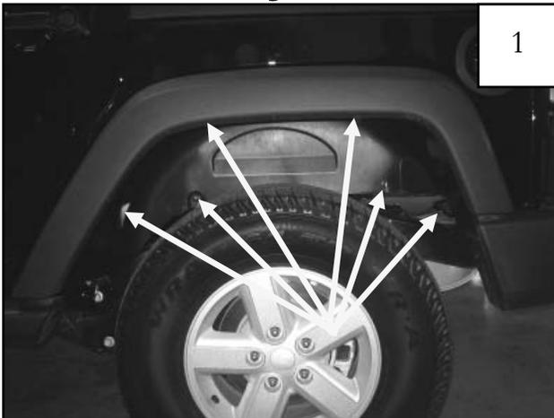
Using a pry tool, pliers, or flat head screwdriver, remove the six plastic fasteners from inside of splash shield.
