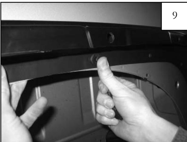
Position Inner Flare Piece on fender, aligning existing 5/16" holes in Inner Flare Piece with holes in fender. Install supplied Plastic Push Retainers (9 places).
