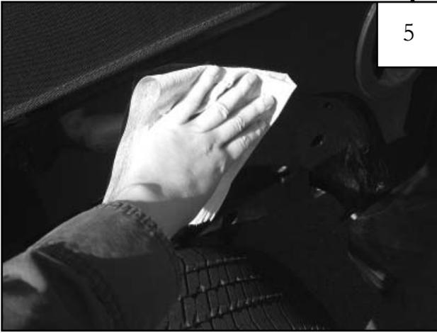
Clean fender area thoroughly with a soft clean cloth and isopropyl alcohol.
